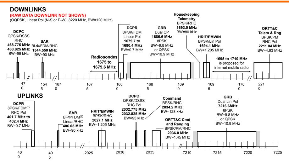
NOTES †: DCPR (8PSK) and SAR (Bi-Φ) are individual uplinks FDM'ed in the spacecraft transponder.
